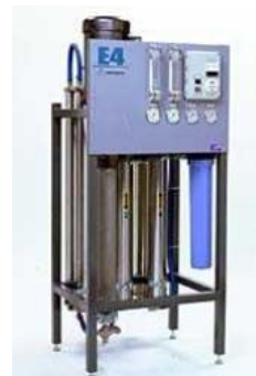
Figure 5: Reverse Osmosis Pilot Unit
