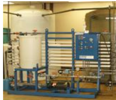
Figure 3: Crown's objective was the successful implementation of a tubular wastewater ultrafiltration system, reducing the amount of waste hauled off-site by up to 95%.
